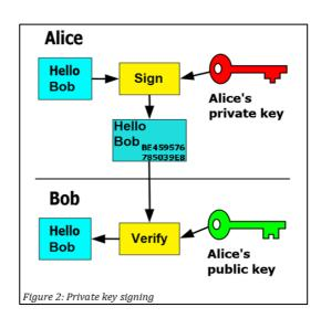
Asymmetric cryptography involves complex mathematics. This would slow down data processing, making it suitable for small amounts of data only. Asymmetric cryptography is therefore often used to generate or exchange symmetric encryption keys<sup>50</sup> (such as the Diffie-Hellman or RSA algorithms).
